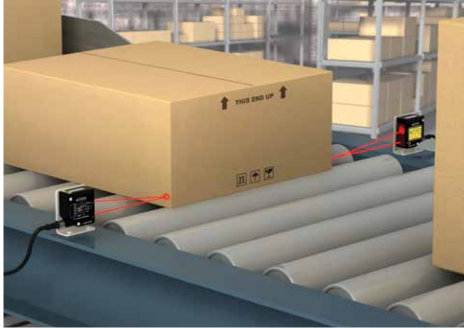
Measuring box width for sorting
