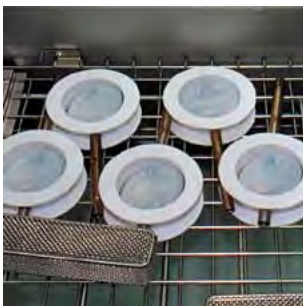
Decontamination by ultrasonic cleaning
