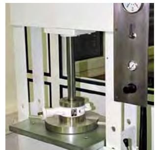
Tightness test with HP nitrogen
