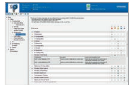
Diagnostic data is categorized or can be user-mapped into five categories according to the severity and ease reactions by the operator. Detailed configuration enables predictive maintenance.
