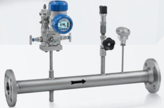
OPTIBAR MR 2000 Calibrated meter run with averaging pitot tube for nominal sizes DN 15...50 / 3/4...2"
